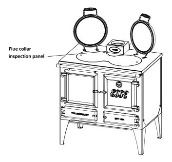
When both the cook stove and chimney are warm, a reading in a range between 1.25mm wg (12 Pa) and 2.5mm wg (25 Pa) should be expected. Any readings significantly outside this range are likely to cause problems, so further investigation should be undertaken so as to either reduce or increase the flue draft reading, as appropriate.
