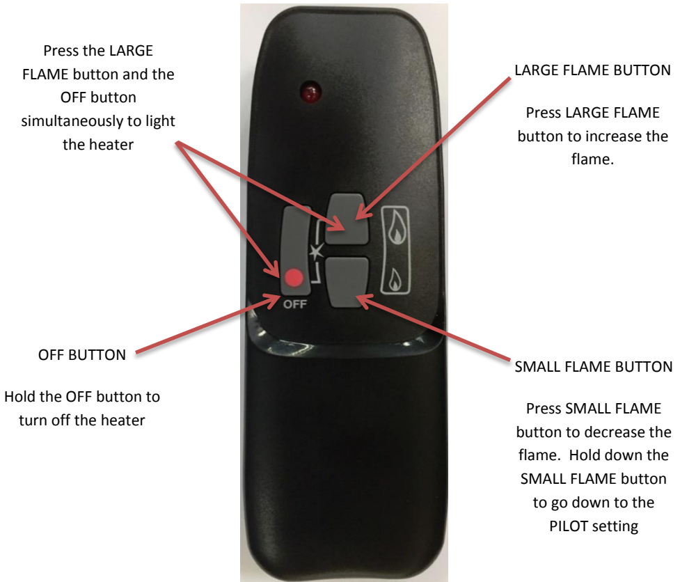
Figure 19 Remote Burner Handset
