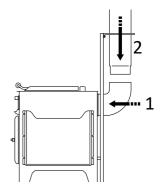
To assemble the flue – insert elbow flue pipe to the rear of the stove and fit the 1000mm length above.
