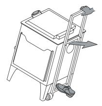
Your ESSE Garden Stove comes supplied with the wheel trolley in position. To move the appliance, place one foot on the base of the trolley, and gently rock backwards, onto the two wheels. You can now carefully pull your ESSE Garden Stove into position.
