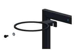
To fasten the halo to the frame use the screw and washer provided. Tighten with the 10mm spanner.
