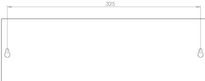
Figure 8 Control Panel Mounting Holes
