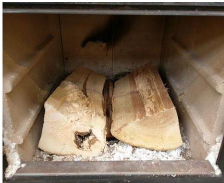
*Figure 11 Logs Laid in Firebox*
