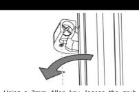
Using a 2mm Allen key, loosen the grub screw on the underside of the handle, by turning anti-clockwise.
