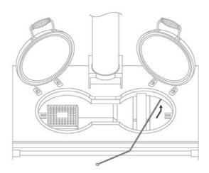
There are two methods to clean the right side flueway. The first is to insert the brush at a shallow angle as shown above. The brush will need to turn 90° into the flueway so steady pressure will be needed to help the brush head round the bend. Once in, work the brush up and down and front to back as the flue way runs along the entire depth of the ovens. Again, soot will fall into the trap between the ovens.
