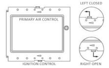
Open the outer cast iron door to reveal the glass door and set primary and ignition air controls to open position.
