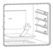
FIGURE 21: USE THE FLUE RAKE TO PULL ANY SOOT OR GRANULES INTO THE OPEN SPACE TO BE VACUUMED.
