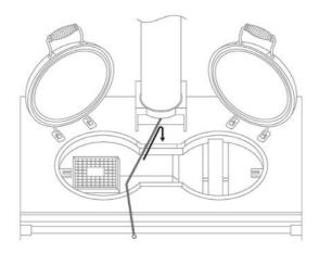
Remove the front of the flue connector box and insert the flue brush from left to right, angling the brush down at 45°. Once you find the flue way entrance push the brush down until it stops then gently but firmly pull back and forth 3 or 4 times then remove the brush. Dislodged soot will fall into the tray between the ovens.
