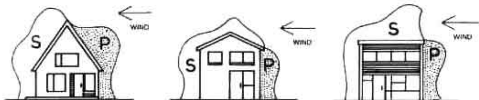
Fig. 6 – PRESSURE AND SUCTION ZONES CREATED BY WIND
