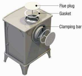
Fig.7 Fitting the fuel bar
